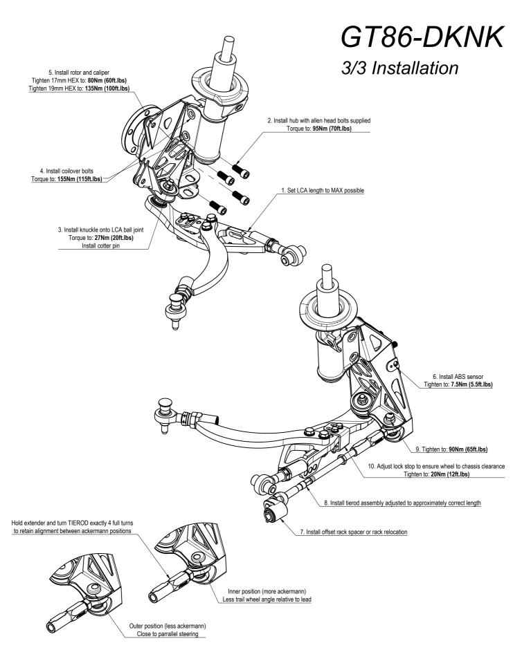
11. Check clearance at full lock through the full range of suspension travel for interference and adjust setup accordingly.
