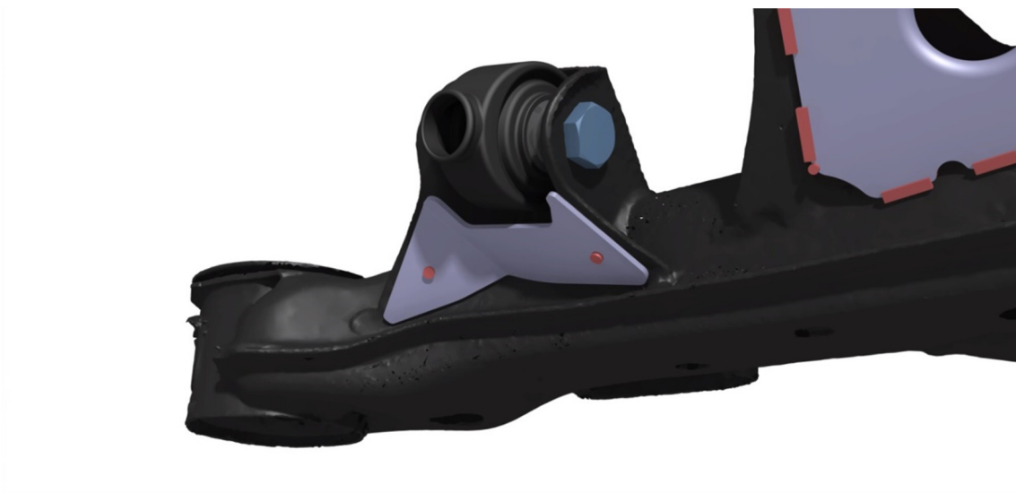
Image 10. Lower control arm front bracket brace plug welds
