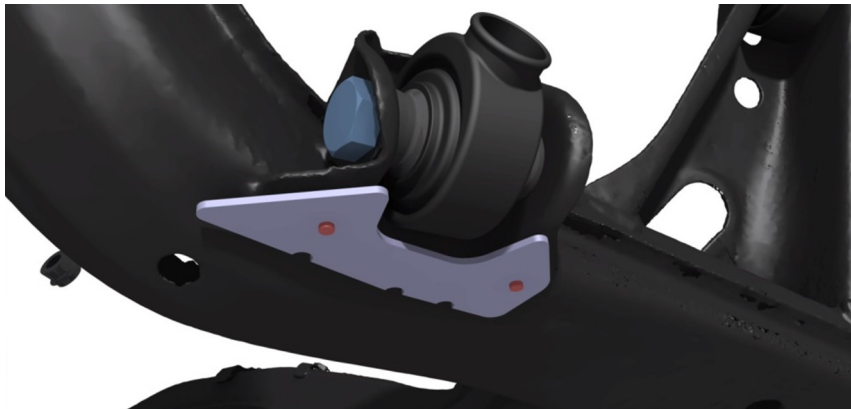
Image 7. Lower control arm rear bracket brace plug welds
