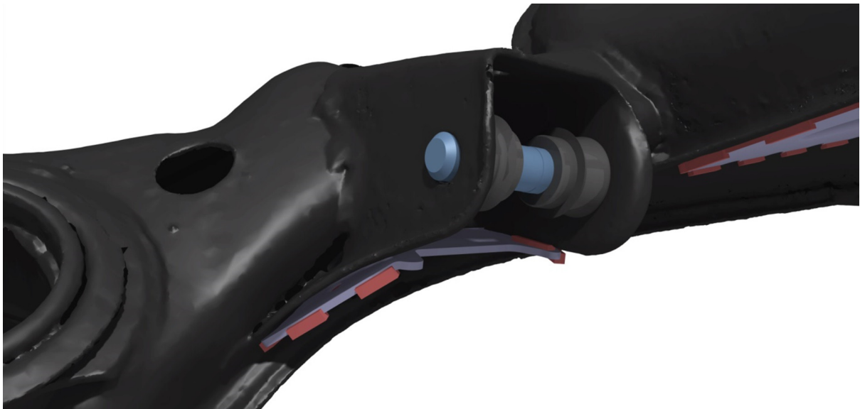
Image 12. Lower control arm front bracket brace inner stitch welds
