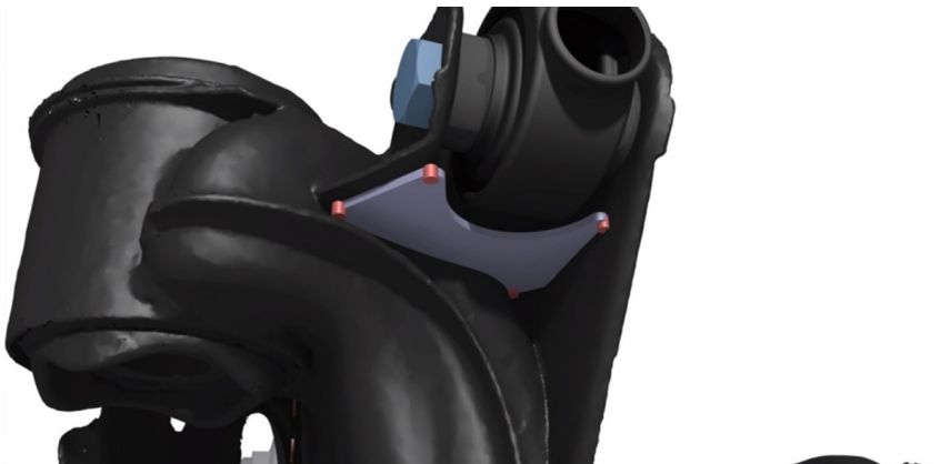
Image 3. Camber arm brace spot welds
