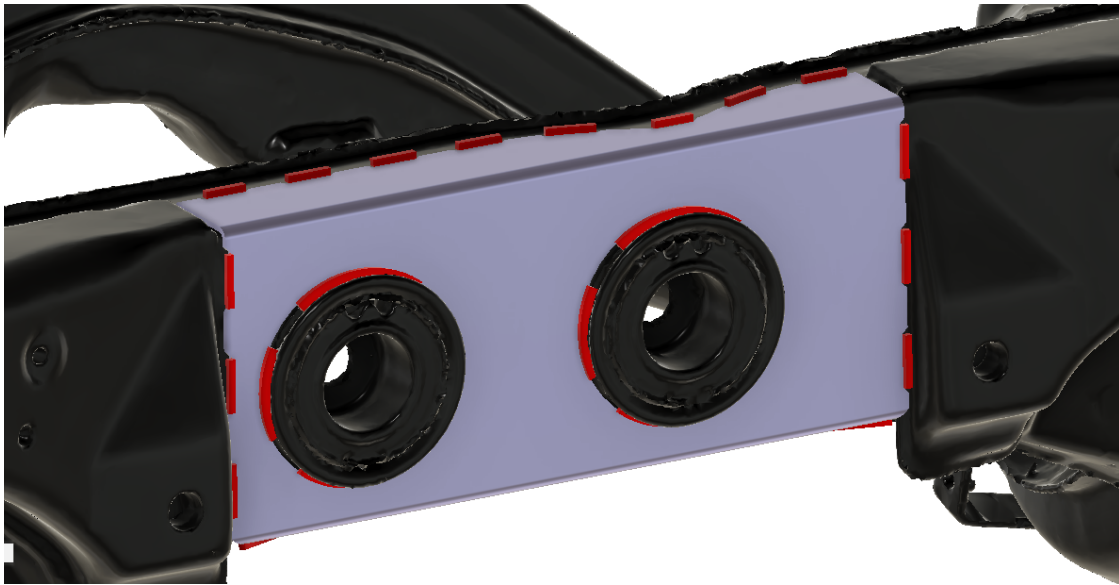
Image 2. Rear differential carrier's brace welding
