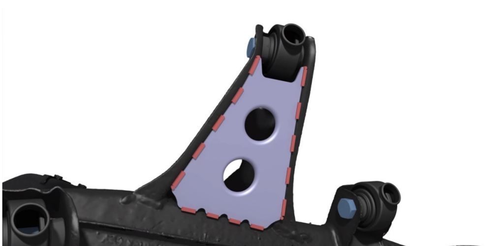
Image 6. Traction arm brace stitch welds
