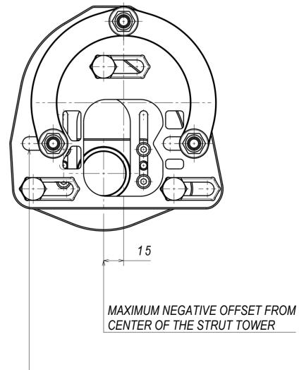
NOTICE THAT CHASSIS MOUNTING HAS ALSO BEEN ADJUSTED FOR MAXIMUM RANGE
