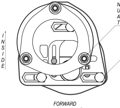
NUT HOLDING COILOVER UPPER MOUNT+CAMBER/CASTER ADJUSTER PLATE, LOOSEN NUTS TO ADJUST CASTER ANGLE FURTHER
