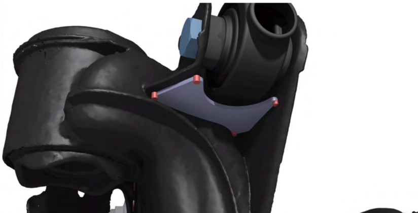
Image 3. Camber arm brace spot welds
