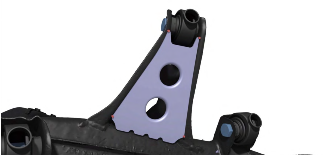
Image 5. Traction arm brace spot welds
