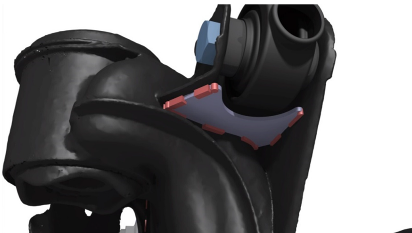
Image 4. Camber arm brace stitch welds
