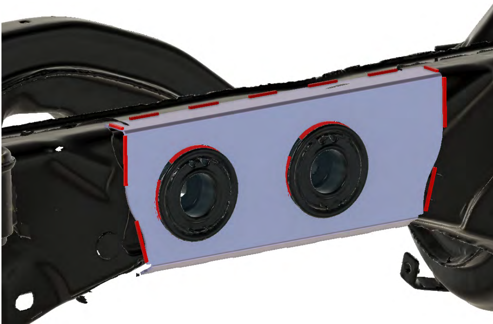
Image 2. Rear differential carrier's brace welding
