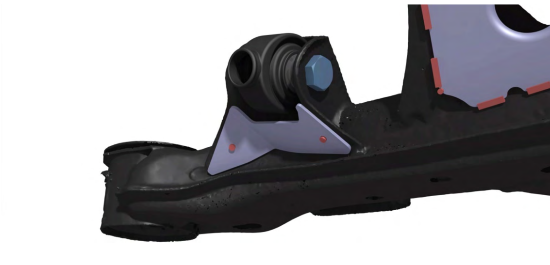
Image 10. Lower control arm front bracket brace plug welds
