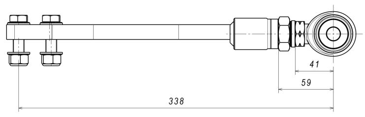
S13 MINIMUM LENGTH - 338 mm S14 MINIMUM LENGTH - 360 mm (MEASURED BETWEEN HOLE CENTERS)
