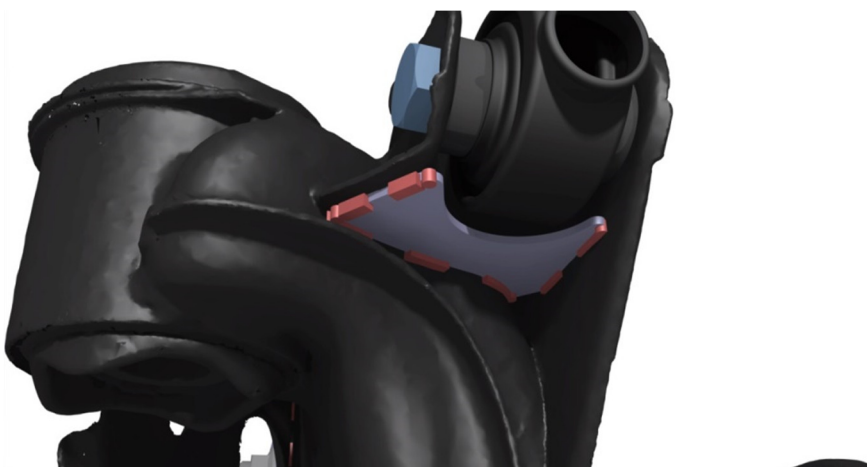
Image 4. Camber arm brace stitch welds
