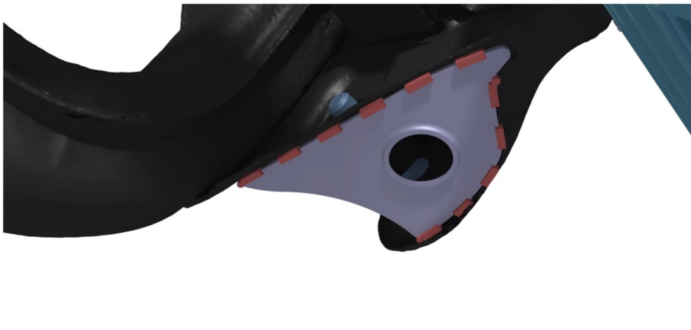
Image 14. Toe control arm bracket brace stitch welds
