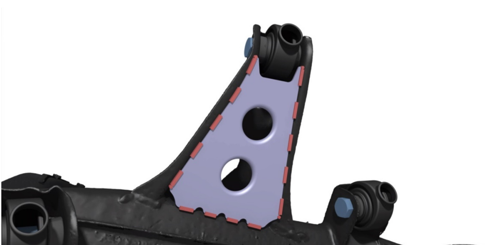
Image 6. Traction arm brace stitch welds
