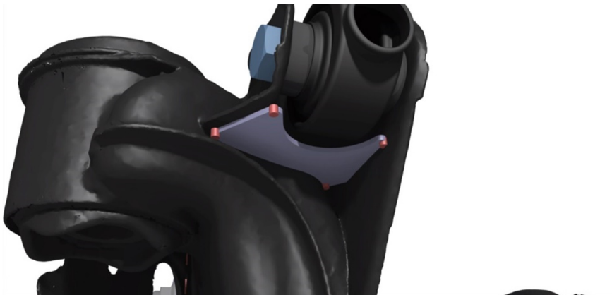
Image 3. Camber arm brace spot welds
