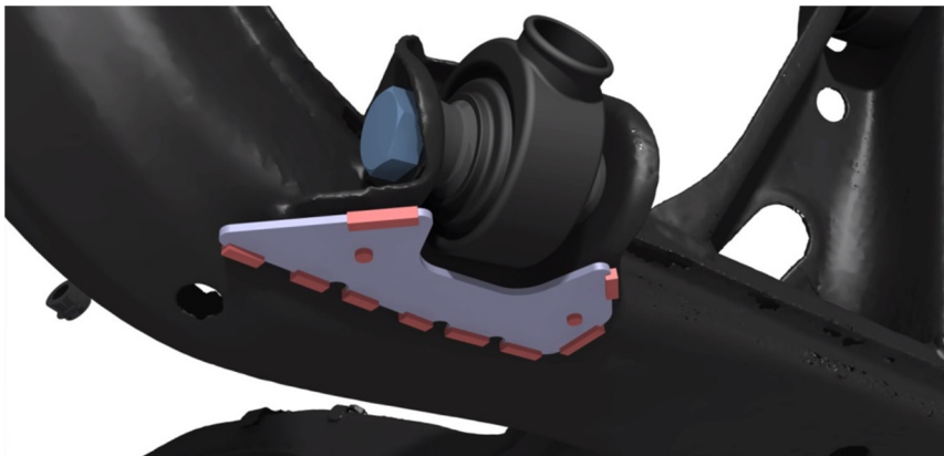
Image 8. Lower control arm rear bracket brace stitch welds
