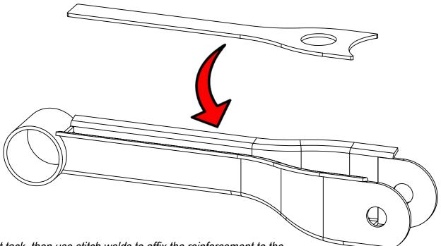
3. First tack, then use stitch welds to affix the reinforcement to the traction rod at the locations highlighted below.
