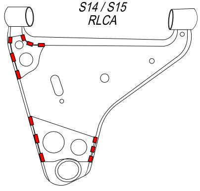
4. Paint the RLCA's to inihbit rust and corrosion, then reinstall in the vehicle.
