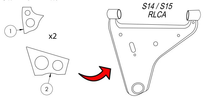
3. Following the completion of the tack welds, the remainder of the stitch welds can be completed at the locations highlighted below.
