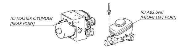
2. REMOVE 2x MOUNTING NUTS TO LOOSEN ABS UNIT. LIFT UNIT TO ACCESS THE FIREWALL LOOM GROMMET.
