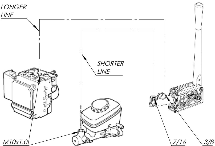
4. CRITICAL - CABLE TIE LINES SO THEY DO NOT INTERFERE WITH PEDALS!
