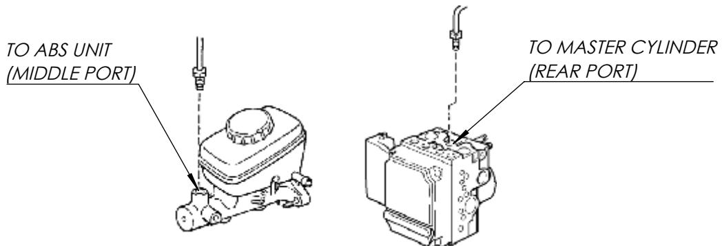
2. REMOVE 2x MOUNTING NUTS TO LOOSEN ABS UNIT. LIFT UNIT TO ACCESS THE FIREWALL LOOM GROMMET.
