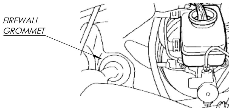
3. CUT A SMALL SLIT INTO THE GROMMET. ROUTE THE LINES AS SHOWN BELOW:
