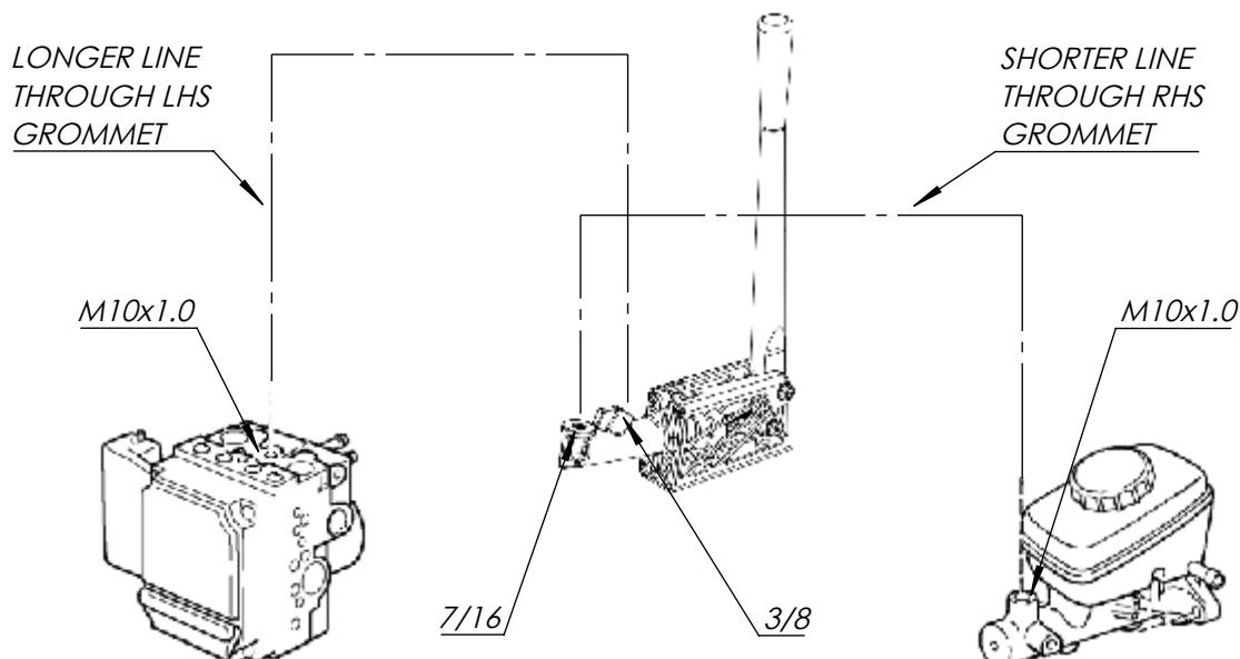
5. CRITICAL - CABLE TIE LINES SO THEY DO NOT INTERFERE WITH PEDALS!
