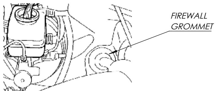
3. REMOVE 2x MOUNTING NUTS TO LOOSEN ABS UNIT. LIFT UNIT TO ACCESS THE FIREWALL GROMMET AND CUT A SMALL SLIT INTO IT.
